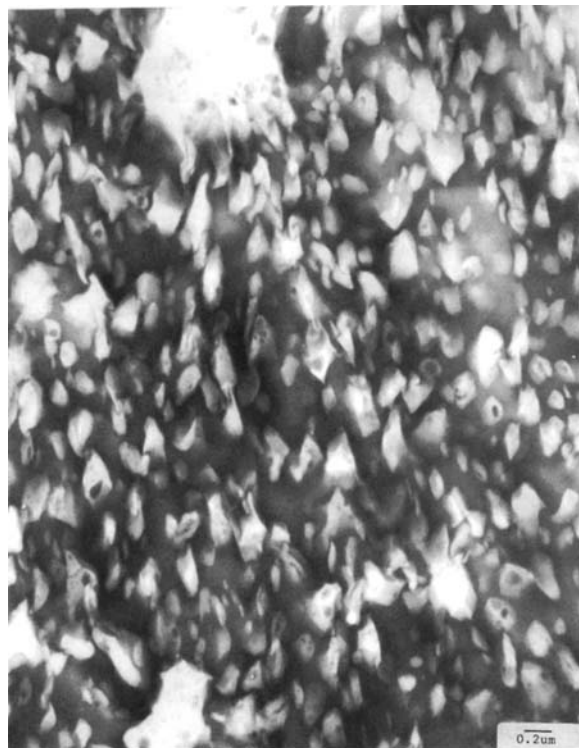
Figure 13 TEM microphotograph of injection molded sequence I ternary blend Z-330/N6/EPX : 16/64/20.
